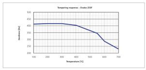
Tempering response for Ovako 253F. Austenitised at 870°C for 30 min and oil quenched. Tempered one hour at each test temperature
