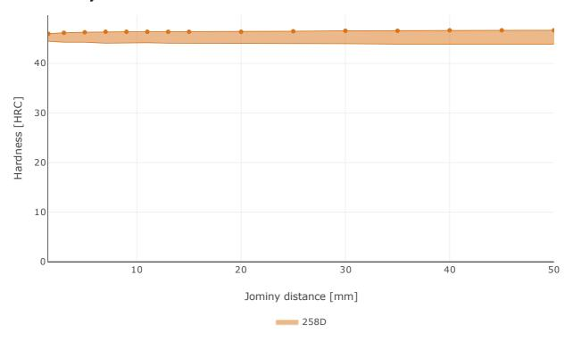
Jominy hardenability according to ASTM A255. Data is average value with +/- standard deviation.
