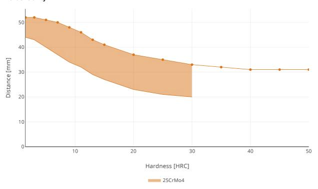
Jominy hardenability according to ASTM A255. The graph shows the average values and standard deviation for 225A and range for 25CrMo4 according to EN 10083:2006. Same graph also valid for 225C.
