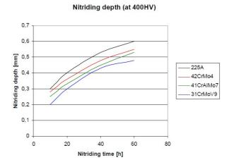
Nitriding depth, defined at 400HV versus process time for different nitriding steel grades. Plasma nitriding at 510°C. Same graph also valid for 225C.
