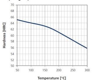
Tempering response for carburized surfaces of Ovako 146S after quenching and tempering one hour at different temperatures.
