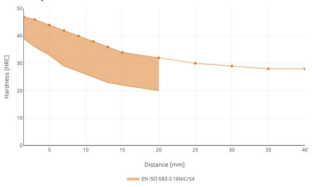
146S: Jominy hardenability according to ASTM A255. Average value with +/- standard deviation.
