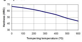
Tempering response for Ovako 825B. Austenitized at  $860^{\circ}\text{C}$  for 30min and quenched in oil. Tempered one hour at each tested temperature
